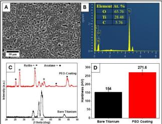
**Fig 1.** (A) SEM micrograph and (B) EDS elemental composition of the optimized coating, (C) XRD patterns, and (D) surface hardness of the bare and coated substrate.
